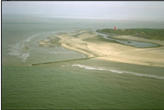
Figure 4-5 Accretion at both sides of a cross-shore dam at the island of Texel (Waddenzee)
