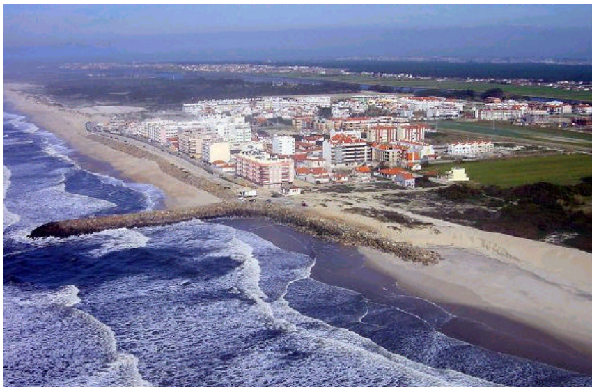
Figure 3-9. The picture illustrates the extent of coastal erosion in Vagueira, located 9 km south of Aveiro harbour entrance. Sediments carried along the coast by longshore currents are partly trapped by the harbour's breakwater, which results in a sediment deficit down-drift and coastal erosion. In the case of Vagueira, the coastal section protected by a rocky structure protrudes of about 30 to 50 meters (with an average rate of 4 meters / year) compared with the non-protected sections. Without protection, the first line of buildings would have collapsed.
