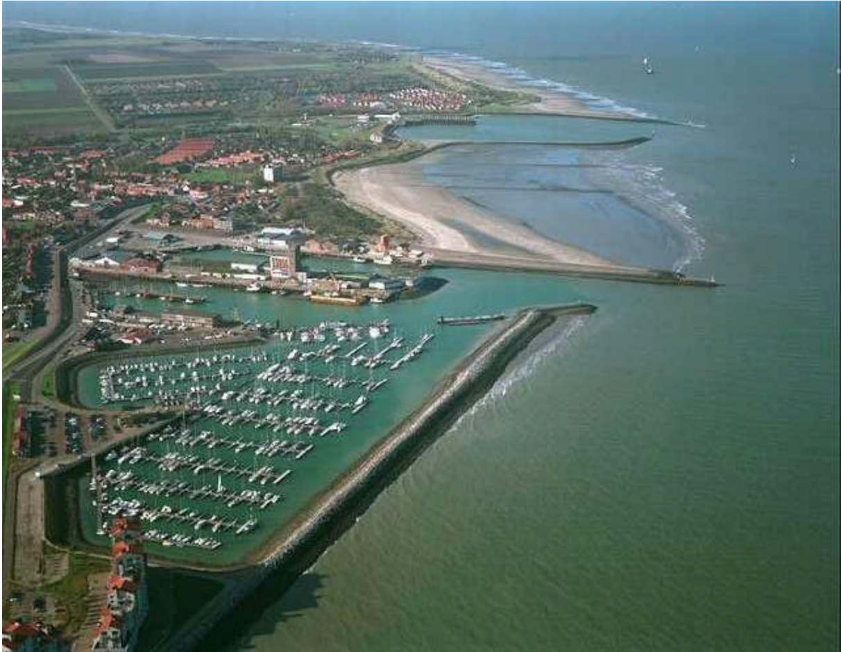
Figure 3-5. The harbour of Breskens is located in the province of Zeeuws-Vlaanderen in the Netherlands illustrates the case of sand trapping by jetties. This photograph clearly shows the accumulation of sand behind the jetties meant to protect the entrance of the marina. This sand accumulation up-drift, results in a sediment deficit down-drift.
