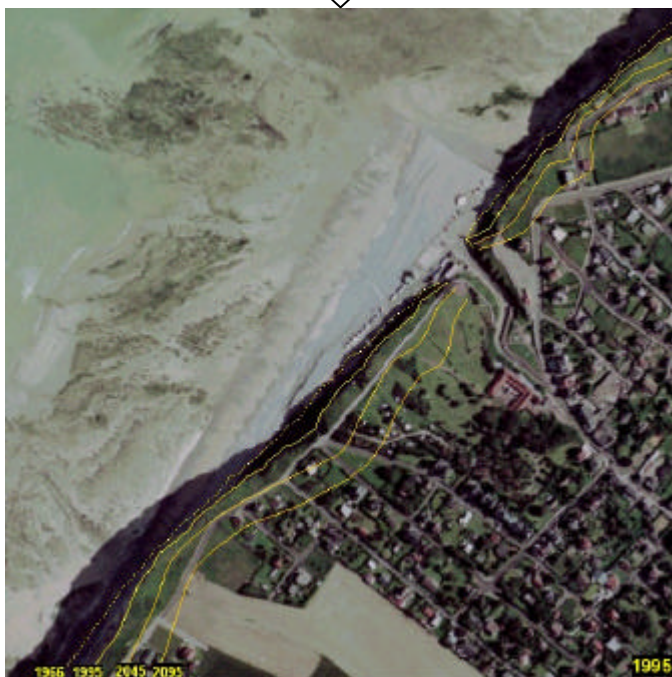
Illustration of a GIS-based local information system dedicated to cliff retreat monitoring and prediction
