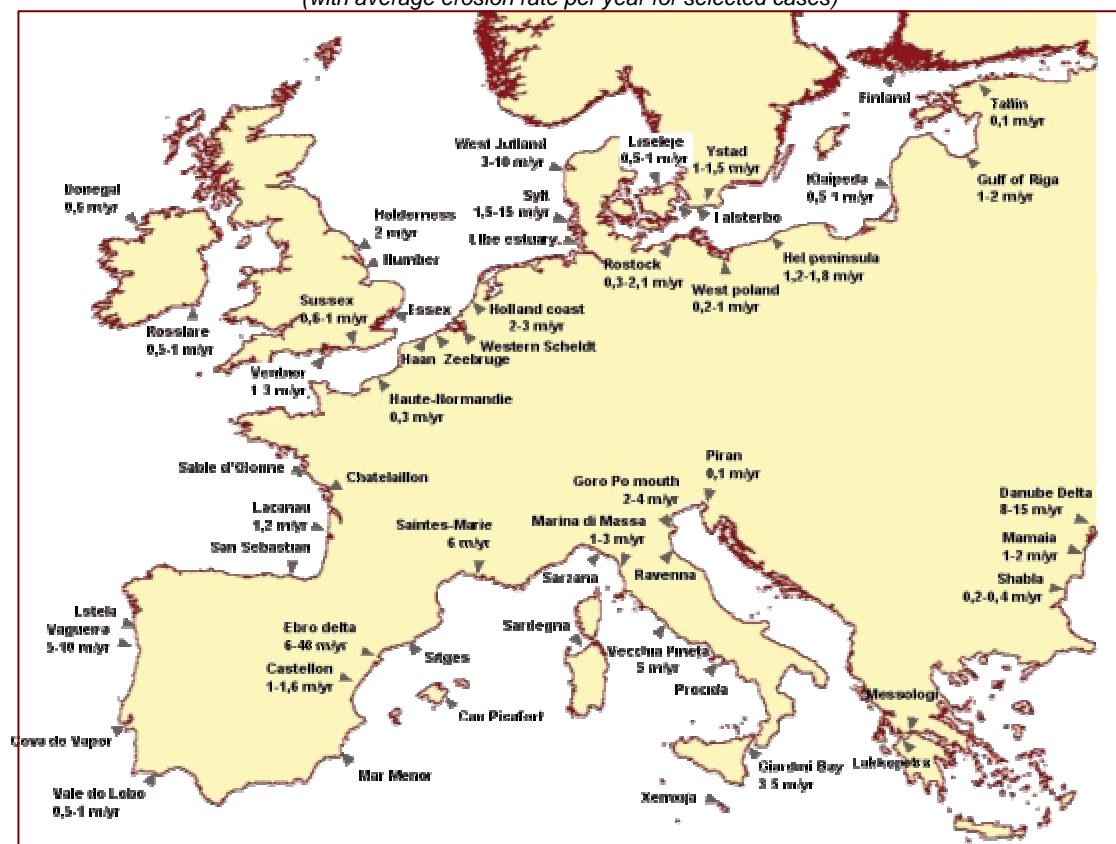
Figure 1. Location of the 60 case studies reviewed during EUROSION study (with average erosion rate per year for selected cases)
